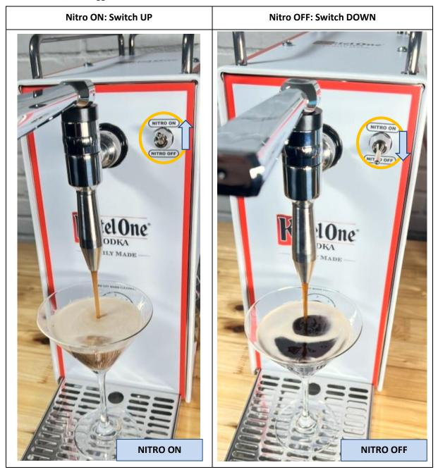
When changing from NITRO-ON to NITRO-OFF it takes about 50 ml (1.7 oz) of product until the remaining nitro gas is out. Open & close the tap handle a couple of times (3-4) and dispense the 50 ml (1.7 oz) in small batches, like this the gas in the tap is flushed out faster.
