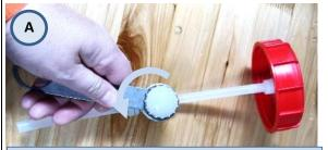
Open filter adapter with wrench Note: Filter adapter might have different position
